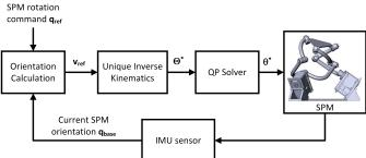
Fig. 3. Block diagram of the SPM orientation control framework.
