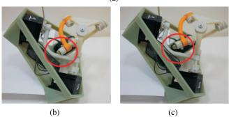
Fig. 7. Inertial stabilization of the Agile Wrist SPM prototype (a); large displacement of the SPM base platform: (b) - the reference  $\Theta^*$  is directly imposed, resulting in link collision; (c) - the constrained reference  $\theta^*$  is used, and collision avoidance is achieved.
