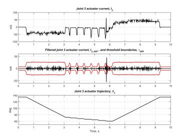
Fig. 4. From top to bottom, time evolutions of, respectively: measured currents of the Joint 3 servomotor (Dynamixel MX-106); high-pass filtered currents (in black) and time-varying threshold (in red); joint position  $\theta_3$ .
