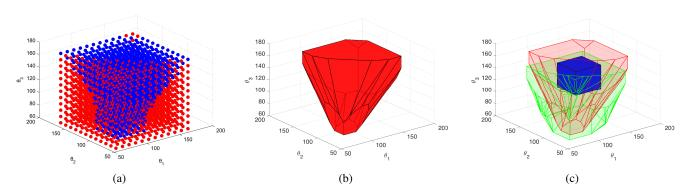
Fig. 5. Estimation of the feasible SPM workspace for the Agile Wrist SPM prototype: (a) - Experimentally obtained SPM configurations, divided into sets  $\mathcal{V}$  (blue) and  $\mathcal{F}$  (red); (b) - Graphical representation of polytope  $\mathcal{P}$ ; (c) - Comparison of  $\mathcal{P}$  (red) with  $\mathcal{S}$  (blue) and with  $\mathcal{P}'$  (green), the latter obtained in [17] for the same SPM prototype.
