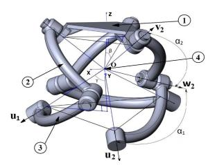
Fig. 1. 3D representation of the kinematic model of a 3-DOF RRR SPM: (1) - top mobile platform, (2) - distal link, (3)- proximal link, (4) - center of rotation.
