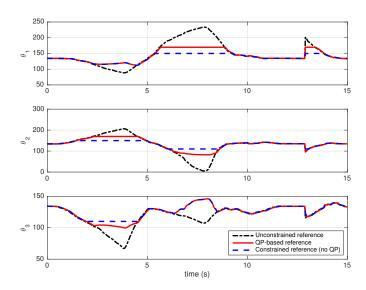
Fig. 8. Experimental time evolutions of signals  $\Theta^*$  (dash-dot black line) and  $\theta^*$  (solid red line) applied to the Agile Wrist SPM prototype for inertial stabilization. Also, the corresponding simulated evolution of  $\theta$  by using workspace S is shown as a dashed blue line.
