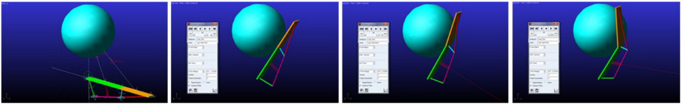
Fig. 7. Simulation carried out on ADAMS showing grasping sequence.
